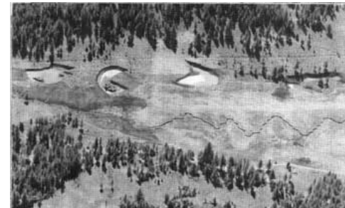
Big Flat meadow after the project. The water has been diverted to the new channel on the other side of the meadow, and the old gully has been converted to ponds
